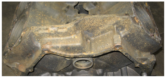
Block casting number location <= 472/500 Block Rear Top View
