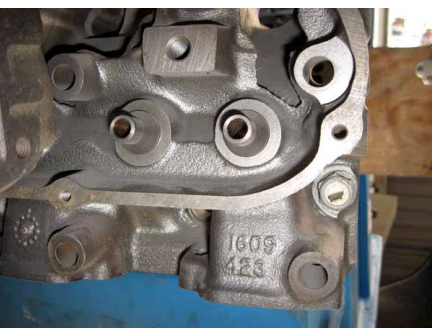
425 Head Casting Number On Exhaust Port
